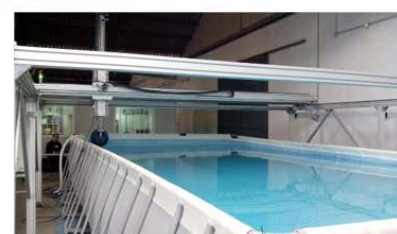
Hydro-acoustic laboratory Tank dimensions 10.0 x 5.0 x 1.5 m 3 .
