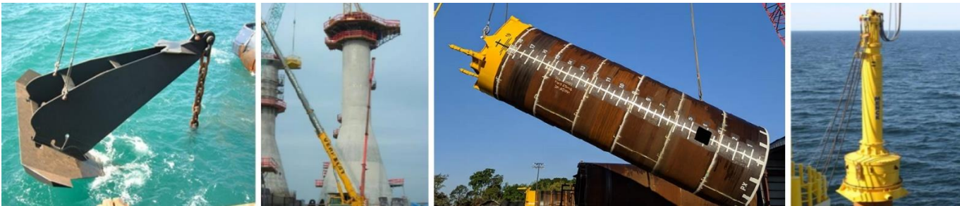
Figure 5: Illustration of the different types of anchors. From left to right: Burial anchor © Vryhof, Gravity anchor © Saipem, Suction piles © Actéon, Pile driver © Menck AG
